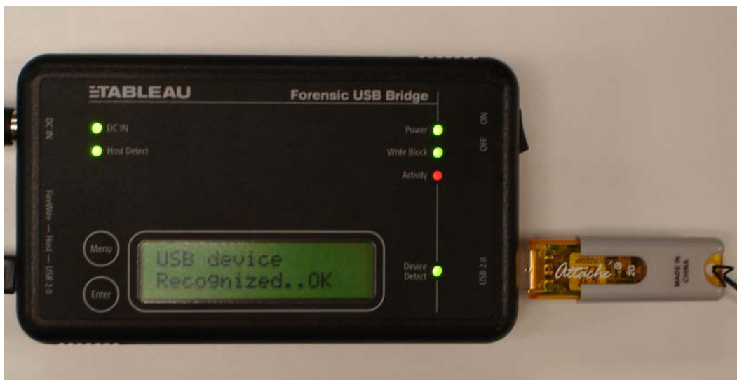
Figure 1.2 2.0 GB USB flash source media attached to Tableau T8 Forensic Bridge
