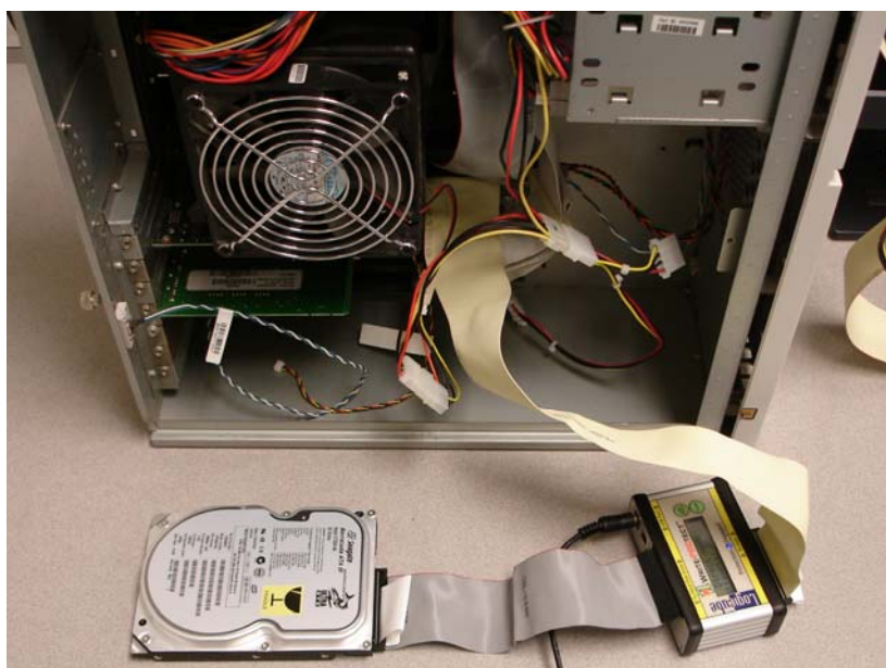
Figure 1.2 - Configuration of test disk drive with attached WritePROtect to the secondary IDE channel of PC
