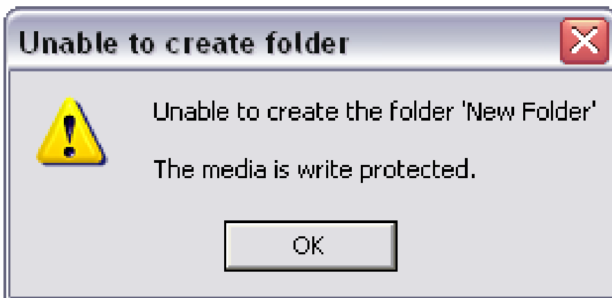
Figure 2.2 Write attempt to USB flash device attached to UltraBlock™ Forensic USB Bridge
