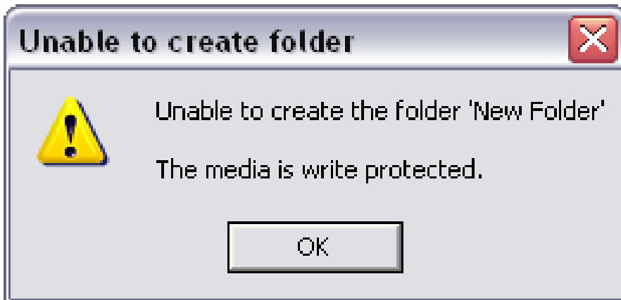
Figure 2.2 Write attempt to USB flash device attached to UltraBlock™ Forensic USB Bridge
