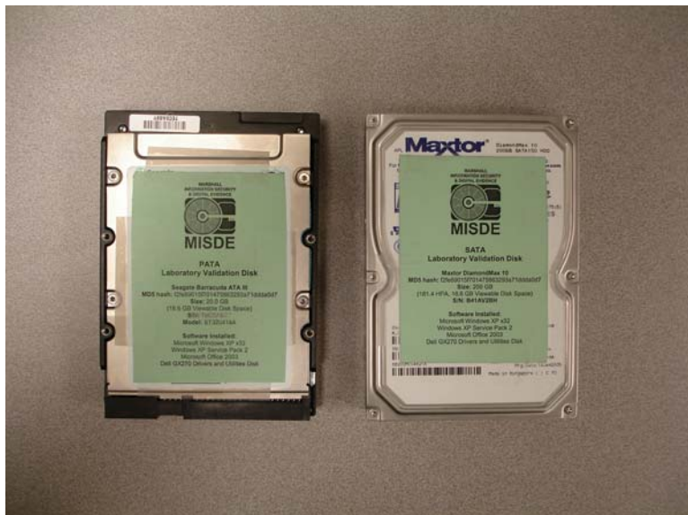
Figure 1.2 Parallel-ATA (PATA) & Serial-ATA (SATA) disks used for testing
