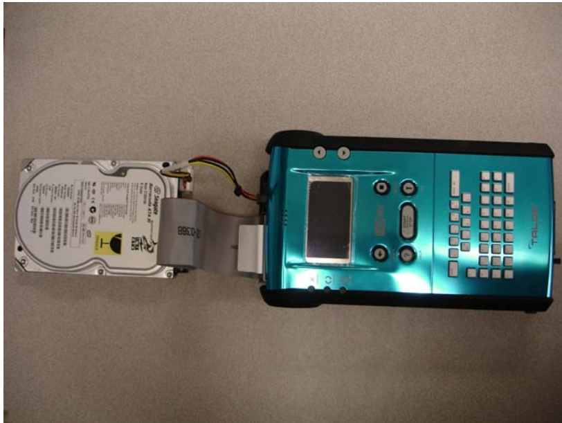
Figure 2.1 18.6 GB PATA disk drive connected to source position
