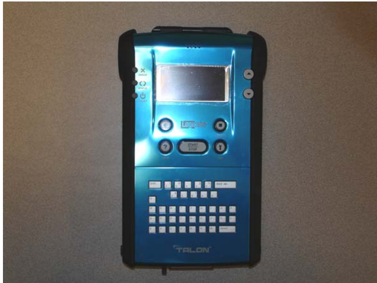
Figure 1.1 Shown is the Logicube® Forensic Talon Capturing System
