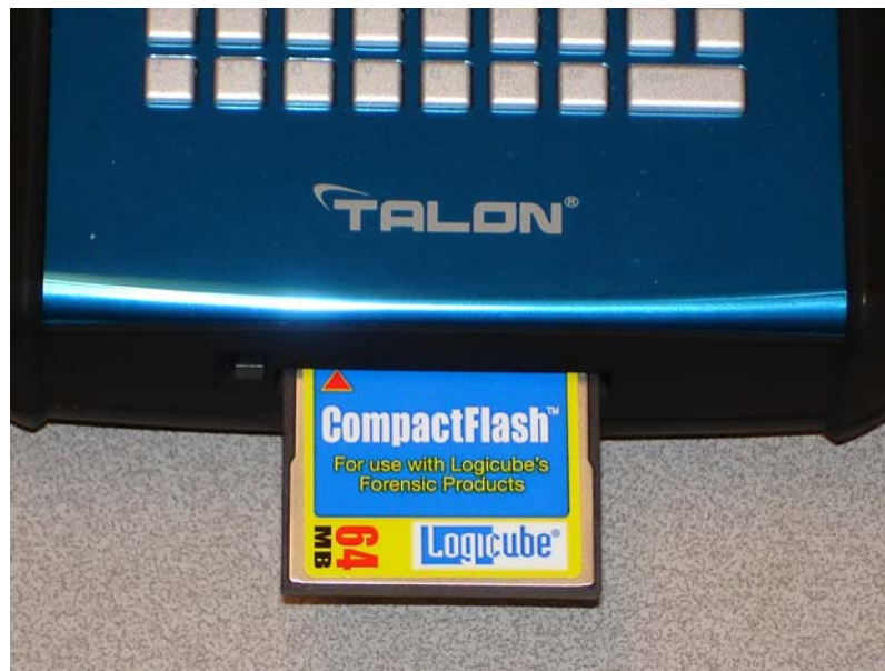
Figure 1.4 64 megabyte (256 MB reported) CompactFlash memory card
